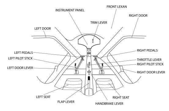
Individual control levers: pilot stick and rudder pedals
